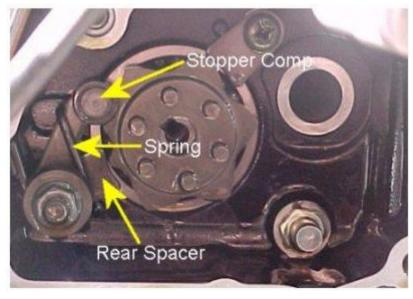
From this point on I am going to call the Stopper Comp the *arm* and I'm going to call the center Shift Gear Cam the *star*. I'm from Oklahoma, I like to keep things simple.
