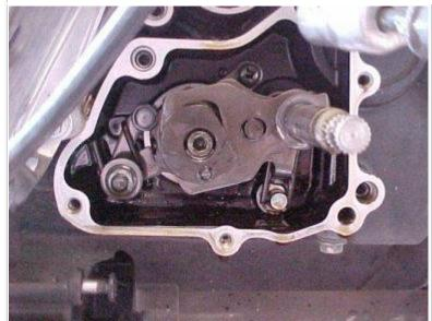
You should now be looking at something like this. There is a snap ring on the shaft that you do not need to remove unless you are going to replace the spring behind it. I removed it, turned out I didn't need to, but I didn't know any better. Snap ring pliers are a must if your planning on removing them (Autozone, \$11.99 and took me about 30 minutes to go to town and get them).
