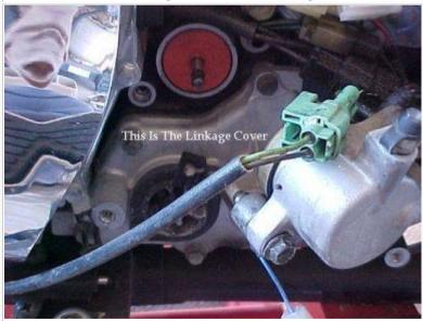
Now that you have the clutch slave cylinder out of the way you can actually get to the cover under which is the shifting parts. Unplug the single wire connector going to the center of this cover (the neutral light circuit) and move this wire out of the way.
