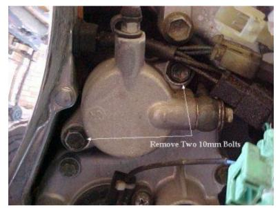
Once you have the secondary cover removed you will need to remove the clutch slave cylinder which can be seen in the picture at left. Some people have removed the lines and fluid but I didn't. Once it was unbolted I simply bunged it over the the side out of my way. You may also have to unplug a few of the electrical connectors to get them out of your way also. Once you have removed the clutch slave cylinder do not squeeze the clutch lever. If you do your going to get brake fluid all
