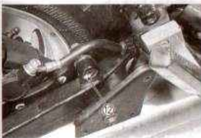
11. Remove the brake caliper holder mounting bolt and nut ⑪.
