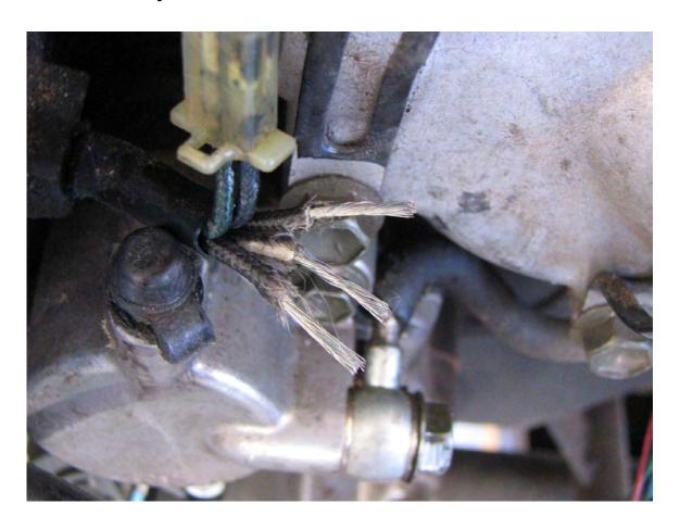
Remove the coupler from the R/R as close as possible to it.
