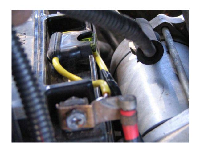
Run the wire from the fuse holder that you just installed and run it down following positive cable from the battery and secure it with a few straps. Do the same for the B/W wire(s) from the R/R and connect to the negative side of the battery **once** you have completed all of the connections.
