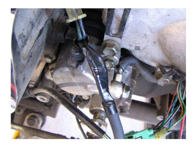
Strip the B/W wire that you already cut off from the R/R coupler and install one eyelet terminal on the B/W wire. The Red wire will no longer be used. Insulate the Red wire so it won't short out anywhere.
