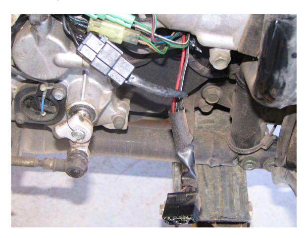
Cut all 3 black wires as close as possible to the Stator coupler.
