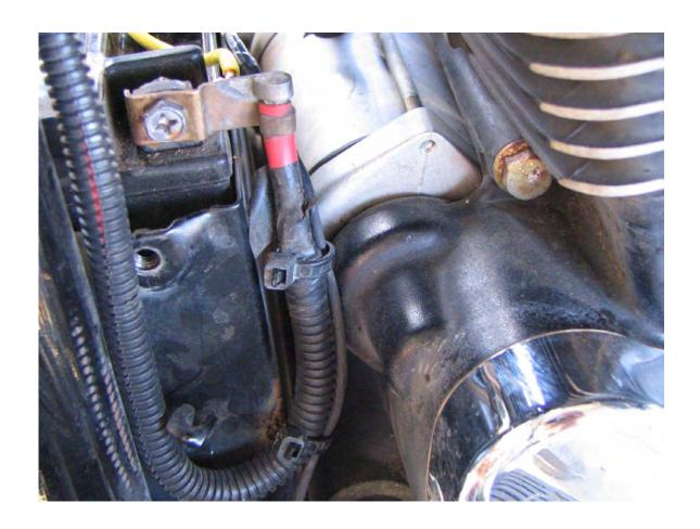
Once all wires are insulated, take the extension cord and follow the frame towards the chrome cover where the R/R was located and follow the wire which comes from the side stand switch which you will see in the next pictures. Once you have the extension cord in position, secure it under the battery box using a strap.
