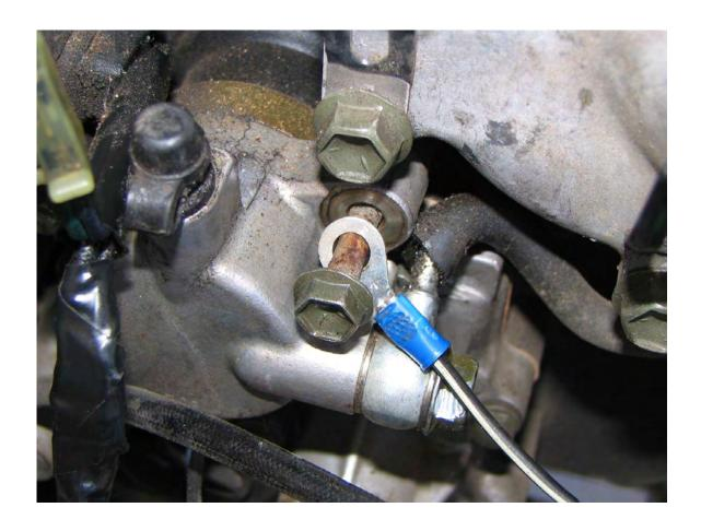
Once you are done these steps, secure all of the wires using the OEM secure clamps and run the newly install Stator extension wire downwards on the left side of the slave cylinder, secure it with a few tie straps and follow the frame towards the battery.
