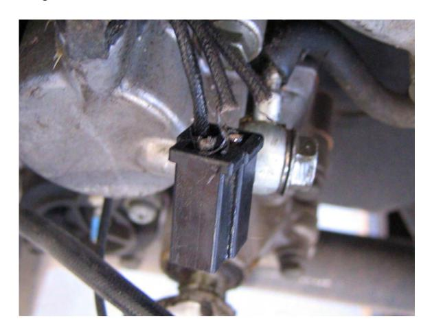
Strip approximately ¾ inch of insulation of each of the 3 black wires. Be careful when stripping the three black wires not to cut any of the wire strands.
