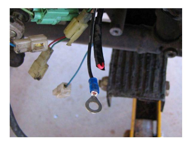
Remove the right hand side hold down bolt on the clutch slave cylinder and install the B/W wire with the eyelet terminal you installed and tighten.
