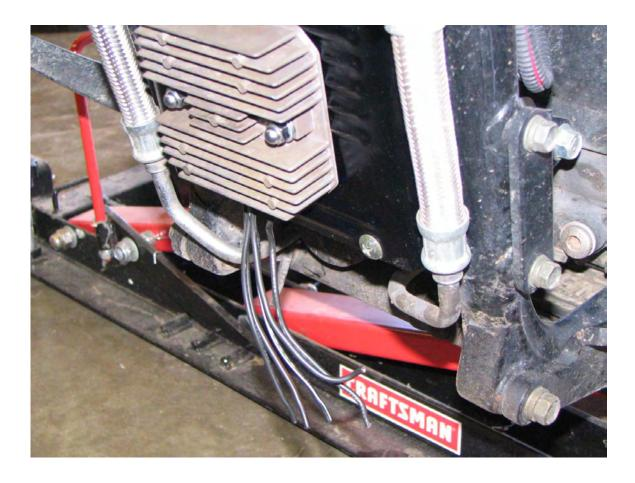
Next, you will need to connect the 3 Black wires from the R/R to the new Stator extension cord. Cut the extension cord, strip the outer insulation and solder them and insulate each one of them. I staggered them to minimize the bulkiness.
