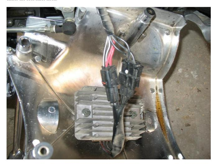
In this picture, you will notice another coupler attach to the R/R coupler. On this coupler, there are black 3 wires coming from inside the left chrome cover. These 3 black wires are directly from the Stator. Disconnect this coupler with the 3 Black wires from the Stator.
