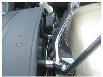
The spacers are PVC pipe cut to the desired length then painted flat black.
