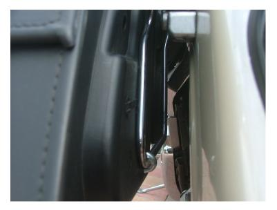
To attach the bottom of the bag to the OEM bracket I just used a U-bolt . The HD mounts had a bar running under the bags to support them from the bottom but I don't load my bags up with that much stuff so I don't need them to carry much weight. You can put another u-bolt up front but will need another spacer to fill the gap. Pics of the inside will show this better.
