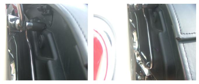
The following pics show the inside of the bags and the position of the mounts and holes drilled. I left the HD OEM rubber grommet in the back mounting hole so you can see the position of the new hole I had to drill to get them positioned right. You can see where the U-bolt attaches on the inside. (I need some washers here!)
