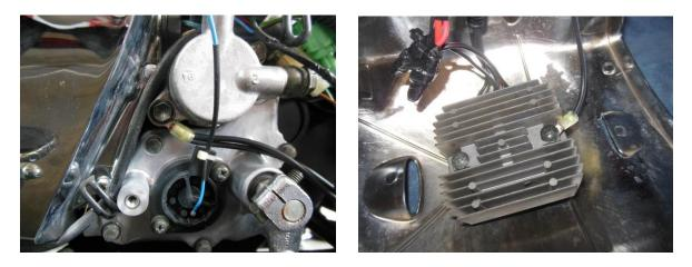
We are literally done with the wires at the regulator area. All your wires should be solid WIRE TO WIRE connections using either solder or secured twist connections. You should have an additional DC Positive (Red) wire connected that runs up to the Starter Relay. And you should have an additional DC Negative(Ground) wire attached to the engine, and optional extra length attached to the Regulator Chassis. The only thing left is the Starter Relay itself.
