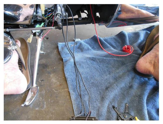
There is a little difficulty while soldering. I didn't have a small torch. You are soldering 12ga wires together. You need patience just to solder 2 12g wires together with a common 40amp solder gun. You need a miracle to solder 3 of them together with the same gun. So, the alternative. Remember, solid WIRE TO WIRE.
