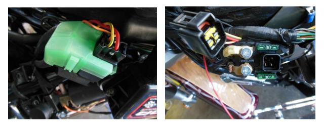
First thing to do here is to remove the fuse from this relay. The one on the top of the above picture is your primary fuse, the bottom one is a spare. Just remove it. It's the same thing as cutting the wire. BUT, by not cutting that wire, if your fuse holder fails (and it DOES happen), you can simply put a fuse back into the relay and get down the road like normal.
