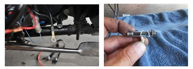
Remove one of your bolts from the shifter mechanism housing. This is where we will be attaching for an additional ground. Place the star lock washer under the head of the bolt, and the ring connector, and put it back in place. The extra ground wire that you added to that ring connector, use one of the regulator mounts for it to act as a chassis ground for the regulator.
