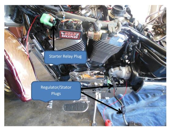
Take note of the red wire I have hanging there. This is the wire we will be using to bypass the starter relay plug. Run it through where you see fit, but try to make sure it's not sitting along something that could melt the casing on the wire. Just let it hang there for now.
