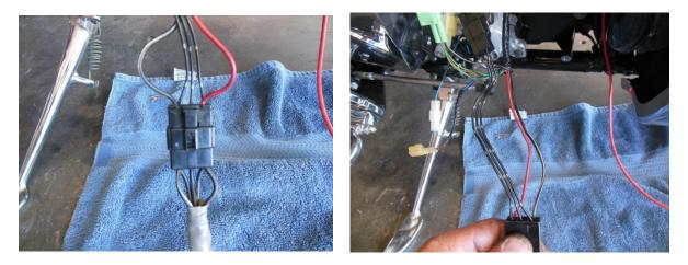
Now for the scary part. Cut those plugs out, throw them away, we won't be using them. You can disconnect the stator plug or simply just cut them all out. So now what we have is simply wires hanging there ready for the hard connection. Note that they didn't give me a lot of room on the stator wires so I tried to point them out. The FEWER connections the better, but sometimes you just have no choice.
