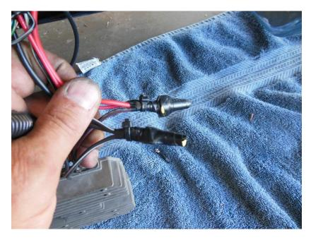
At this point, we have connected all the wires to and from the Stator/Regulator either by solder, or wire twist, with the exception of that DC Negative wire we added (ground). Use one of the ring connectors and attach it to the end of that wire. I also suggest adding another small length of black wire to that ring connector.
