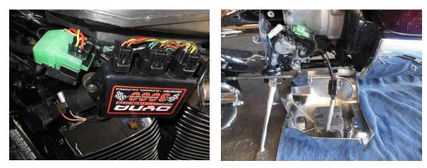
It is safer to remove the regulator from the side cover and place it aside. 2 Phillips Head screws. Below is a picture identifying the 3 points we will be addressing.
