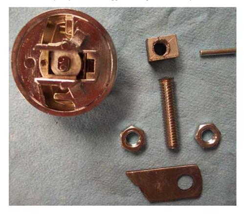
Ok, that 5/16-18 stud will require 9/32 drill bid but I would start with smaller pilot hole and go up may be in 3 steps. When I was installing the stud in the block I used some Red Lock-Tite not to secure it in there but to stop it from rotating while drilling for the Rolled pin. After you insert the Rolled pin in that baby is not turning under any circumstances. Now you see a Bolt that resembles letter T which its head will rest between the EARS on the HD Switch housing. Here is the Pic.
