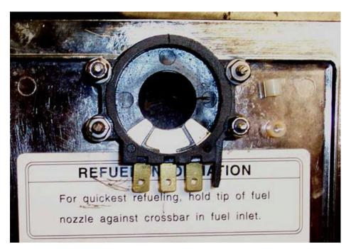
Install center housing, tighten the screws, stick the Black Sticker back on..... nothing will work better than Double sided tape here. During assembly of Switch components use small amount of heavy wheel bearing grease on Tabs and Springs this will retain those Small parts during final assembly also it is good for their proper operation and longevity. After you are done with the Switch, screw in the bottom Jam-Nut then the
