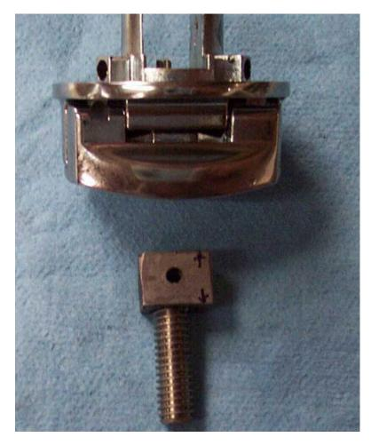
Drill bid size for the Rolled pin depends on what diameter pin you are using, what ever that measurment is, pick a bid 1/32 smaller. This picture will show you where the pin will be installed (drill bid is for demostration).
