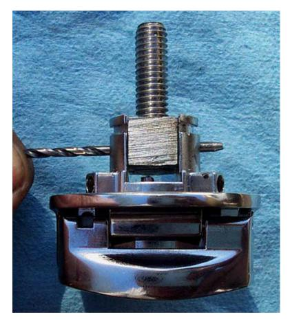
Ok here it is. You have installed the Locking latch and Spring then reseted the block&Stud between Switch's Tabs, then lined up the holes and drive Rolled pin Through. Grind and smoothen both end of the Pin flush with Housing's sides. Now you are ready to set this baby aside.
