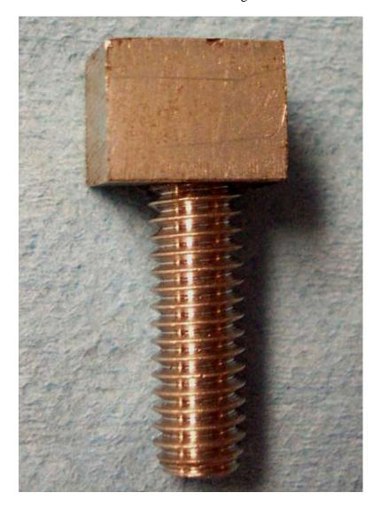
This one will show you the hole for the rolled pin. You insert the Block in the center of the switch housing and drill the hole through all 3 parts at the same time. I removed it after drilling for the Photo only.
