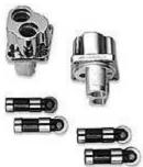
moves further way from the camshaft. How far can a motor grow? Not far but enough to make a difference. Try .040" on an Evo motor, when your valve clearances should be somewhere nearer to .002. With hydraulic lifters, as the engine gets hotter, and the gaps increase, more oil fills the bigger chamber and the slack is taken up.
