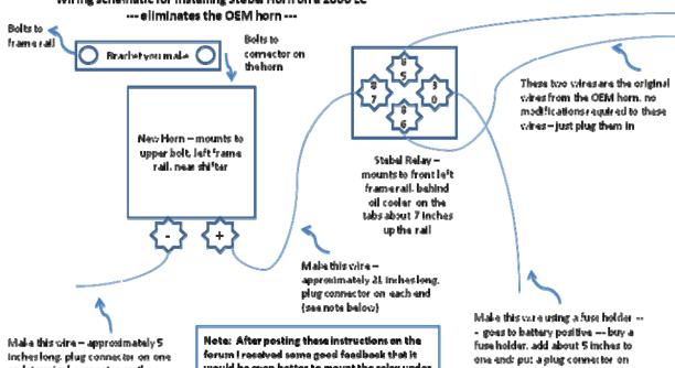
and, terminal connector on the other (big anough to fit the frame) bolt, assuming you are mounting on the frame rail by the shifter)
